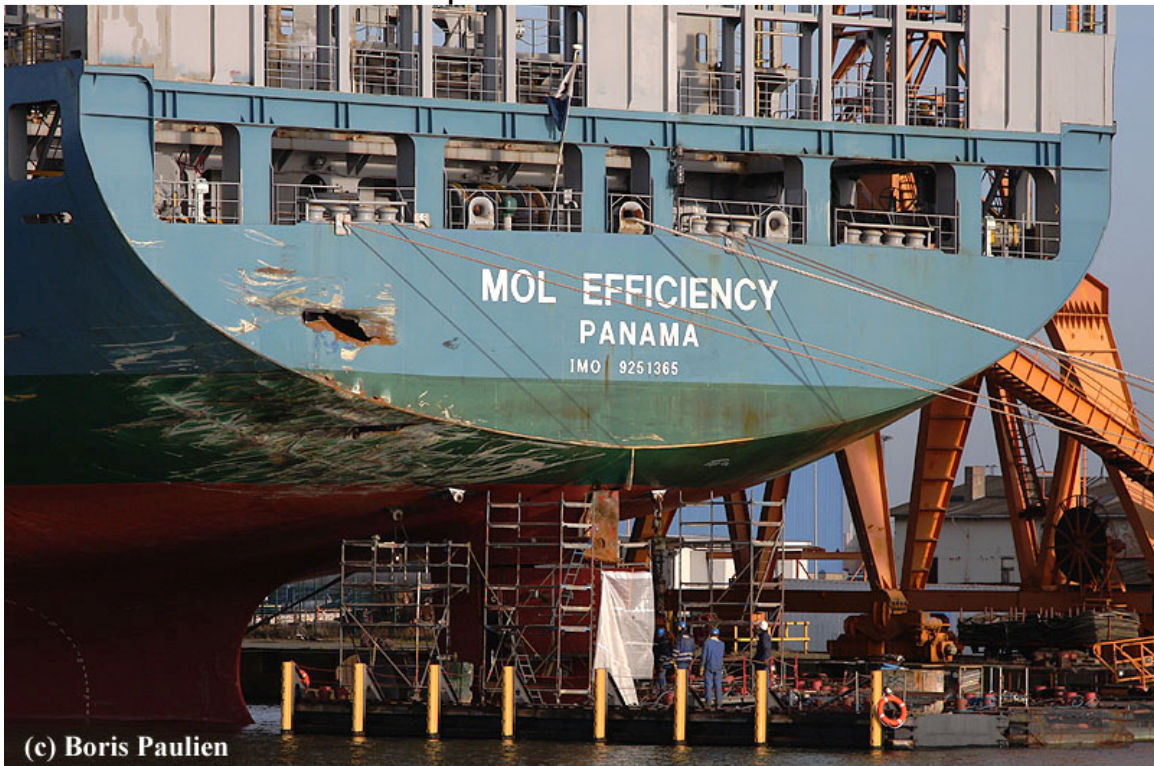
In a collision with a small bulker, MOL EFFICIENCY got holed at Bremerhaven. Here, Lloydwerft carries out repairs on the ship.
