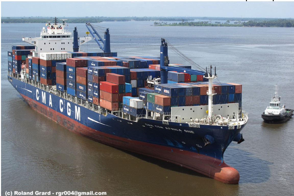
The French Line's geared 3,600 teu ship CMA CGM AFRICA ONE arrives at Abidjan in the Ivory Coast.
