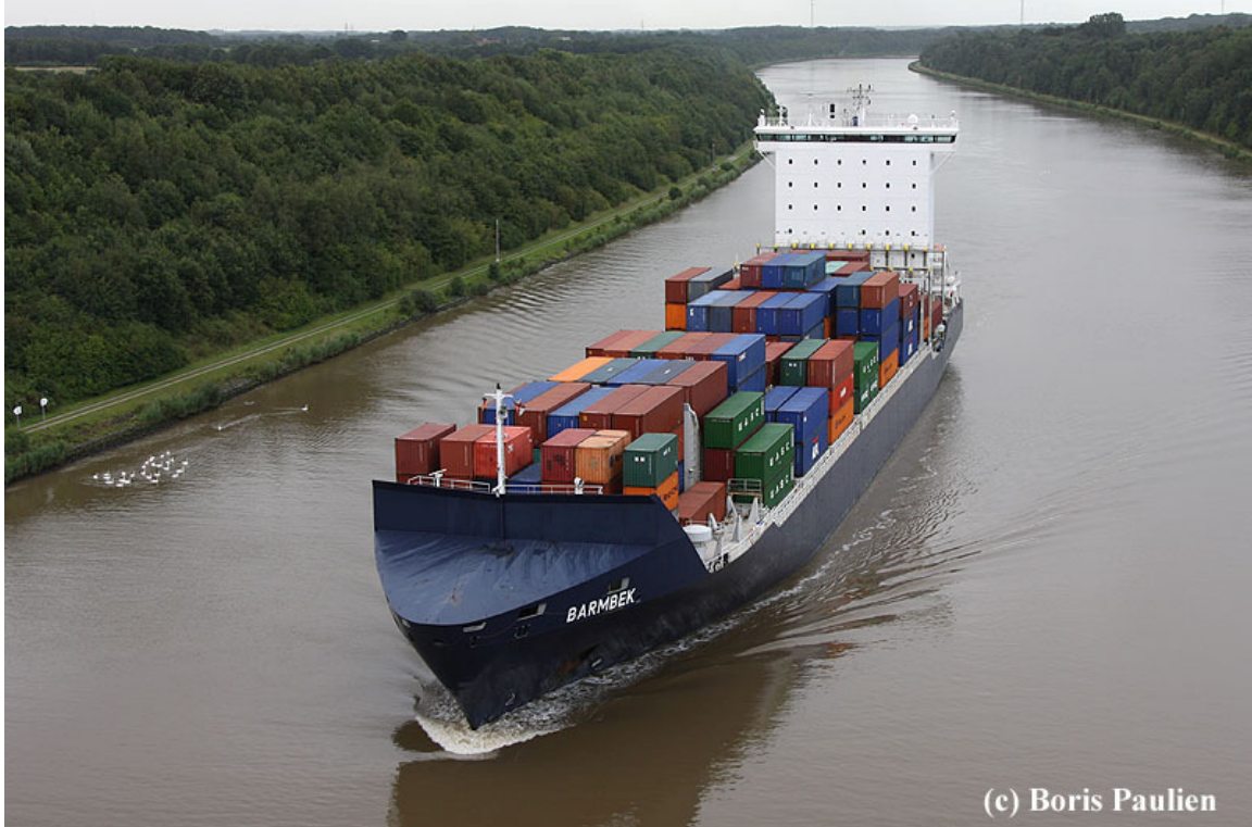
The open-top feeder ship BARMBEK in the Kiel Canal. She is one of four identical container vessel built by the German Meyerwerft.
