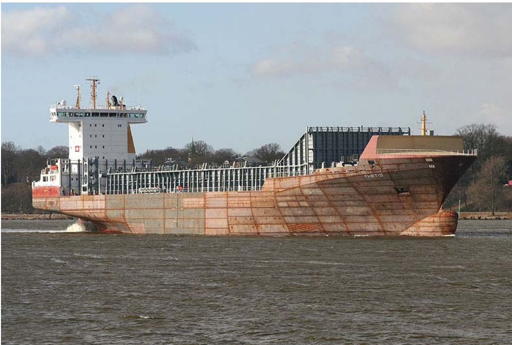
The Sietas-type 178 vessel THETIS at Hamburg: She returns from sea trials with her final paint still missing.
