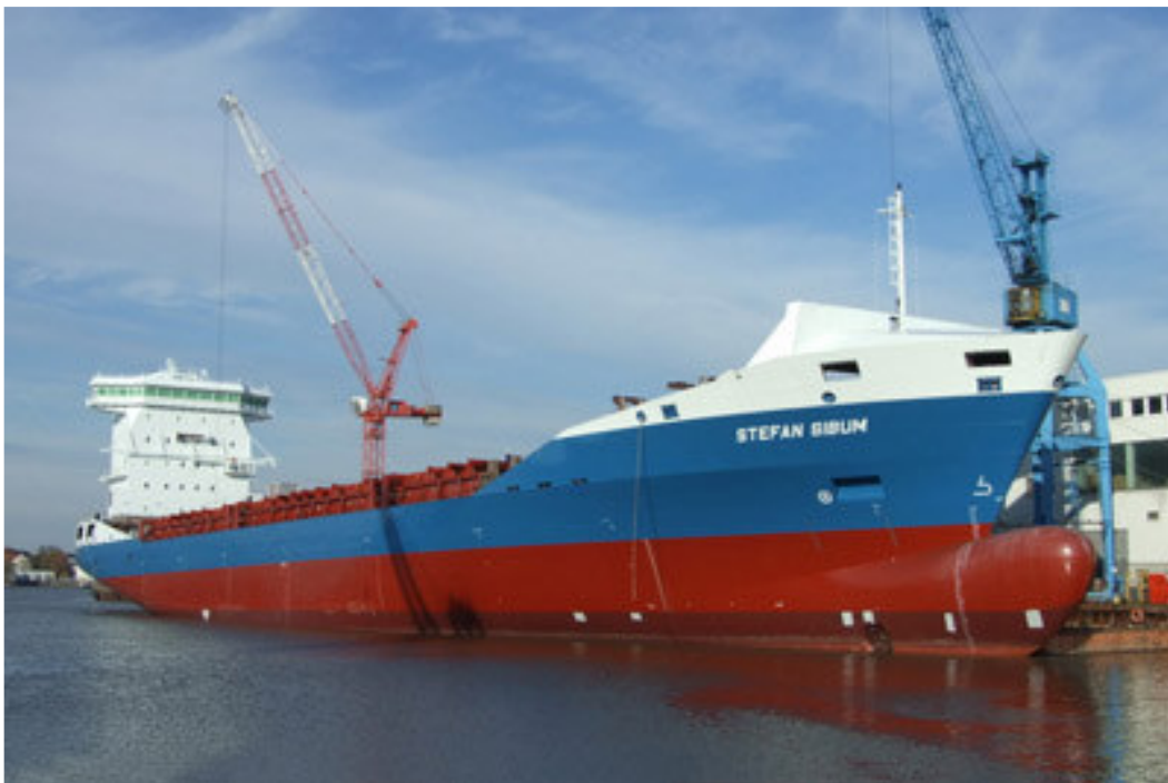
STEFAN SIBUM is seen here at Bremerhaven's SSW yard just after her deckhouse was lifted onto the hull. photographer: Christian Eckardt
