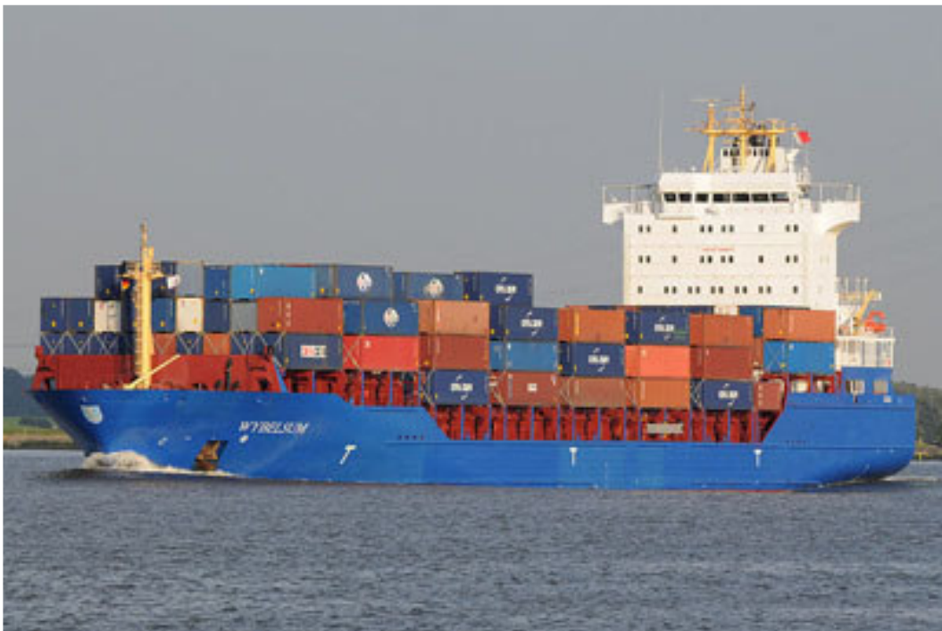
Opposed to her earlier sisters, WYBELSUM is gearless. The Chinese-built Briese ship feeders for CMA CGM. photographer: Michael Witt
