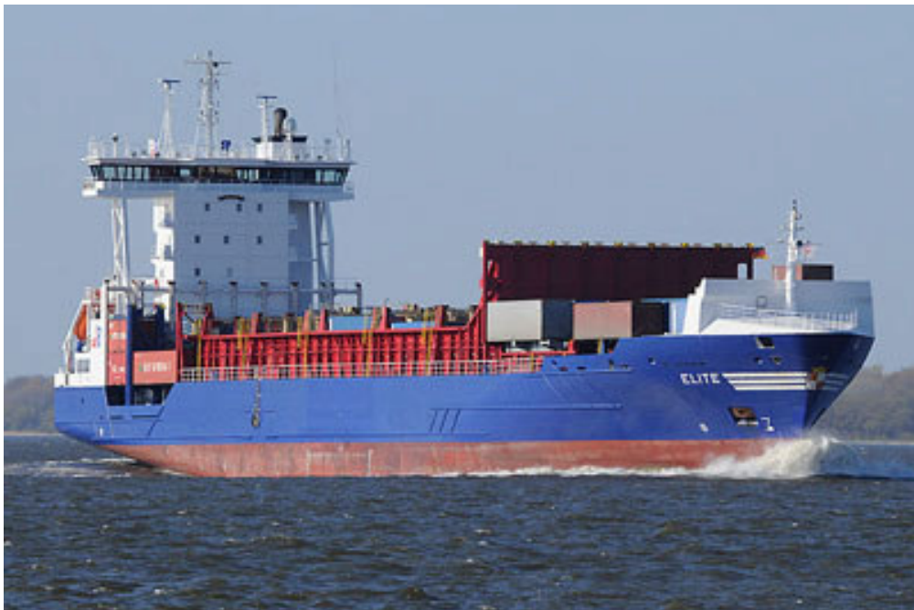
The Sietas-built typ168-feeder Elite has recently been lengthened at Hamburg's Norderwerft.
