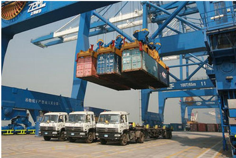
**The gantries can lift up to six TEU or 120 metric tonnes
