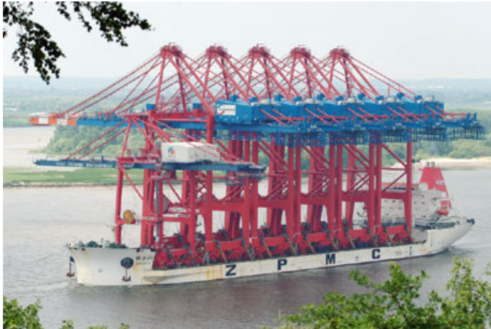
New container handling equipment is being installed at all major ports: Here, a ship with new super post panamax gantries comes into the port of Hamburg. photo: Jan Tiedemann
